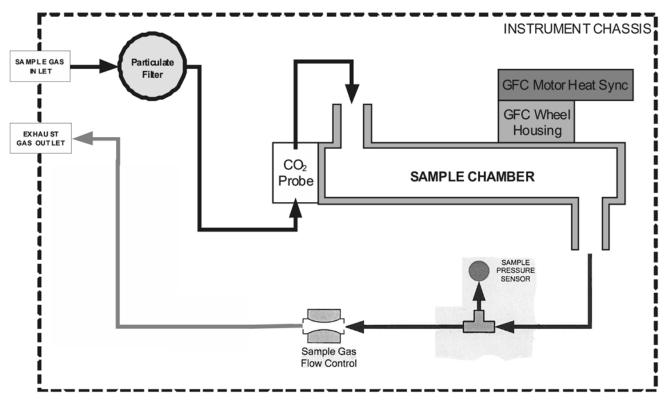
Figure 12-12: GFC7001T/GFC7001TM - Internal Pneumatics with CO<sub>2</sub> Sensor Option 67A
